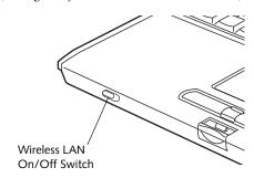
Figure 3. Wireless LAN On/Off Switch
